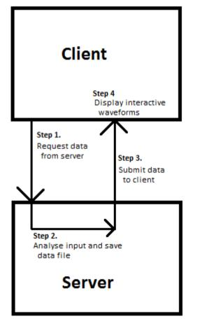
Fig. 1. The client requests data from the server which analyzes the input (VCD file) and returns them in an easy to process format.
