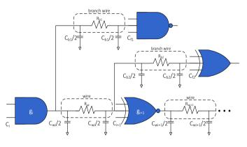
Figure 2 A logic path segment including RC interconnect and two branches
