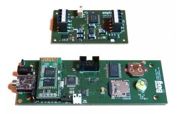
Fig. 6. Miniature strain gauge amplifier (top), autonomous triaxial accelerograph (bottom).
