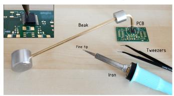
Fig. 2. SMD hand-soldering tools
