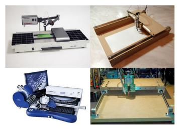
Fig. 4. Commercial (left) and custom (right) manual pick-and-place devices
