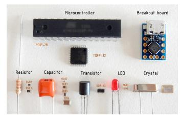
Fig. 1. Surface-mount vs through-hole components and breakout boards
