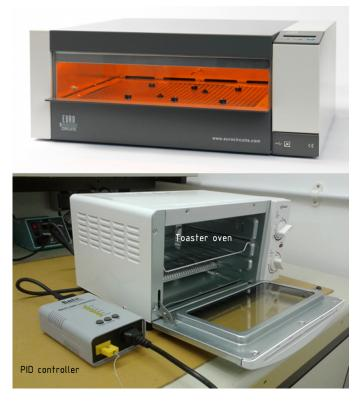
Fig. 5. Commercial (top) and converted reflow ovens (bottom)
