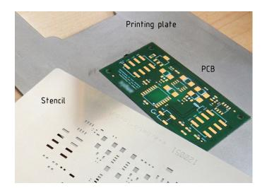
Fig. 3. Manual solder paste printing
